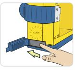
2. To remove the battery, push and move it slightly to the left and then release.
