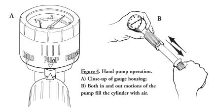
First, rotate the gauge housing of the hand pump to the "PUMP" position. Begin SLOWLY pumping air into the cylinder by stroking the pump handle all the way out and all the way in. Observe the gauge to make sure you are staying within the guidelines provided by your health care provider. DO NOT OVER-INFLATE.
