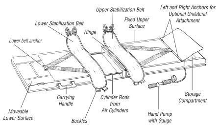
Figure 5. Components of the Saunders STx Lumbar Traction Device.
