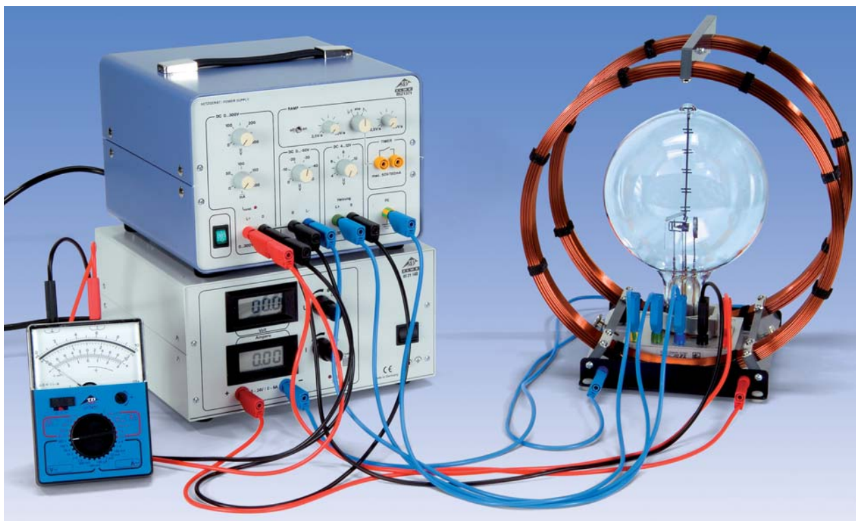
Fig. 2: Experiment set-up for determining the specific charge of an electron
