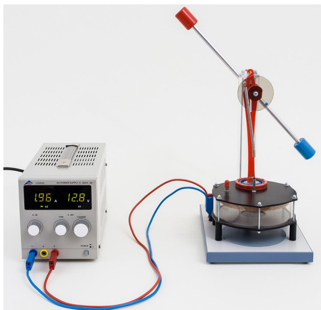
Fig. 5: Set-up for the operation of a Stirling engine as a heat engine by means of electric heating
