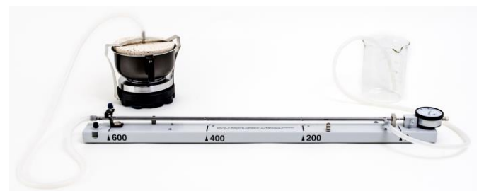
Fig. 12: Set-up with steam generator
