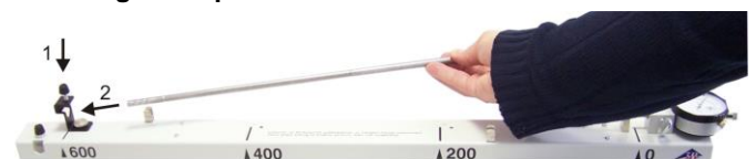
Fig. 6: Attach the fixed bearing to the linear expansion apparatus at about marking 600 using the knurled screw. The steel sample tube should be laid on the apparatus with its open end on the fixed bearing.
