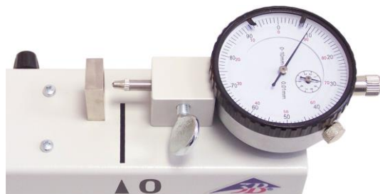
Fig. 5: Insert the gauge fully into the adapter and secure it in place with the wing nut.
