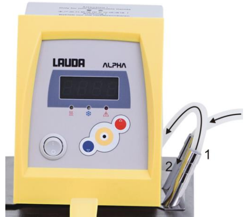
Fig. 10: Feed (1) and return (2) for the pump recirculation set.
