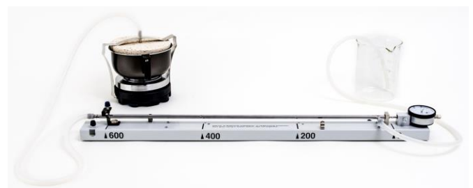
Fig. 12: Set-up with steam generator
