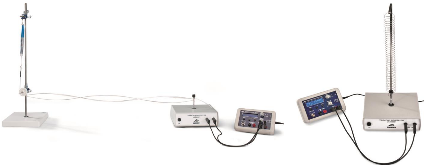
Fig. 1: Measurement set-up for investigating standing waves along a taut rope (left) and a stretched coil spring (right)
