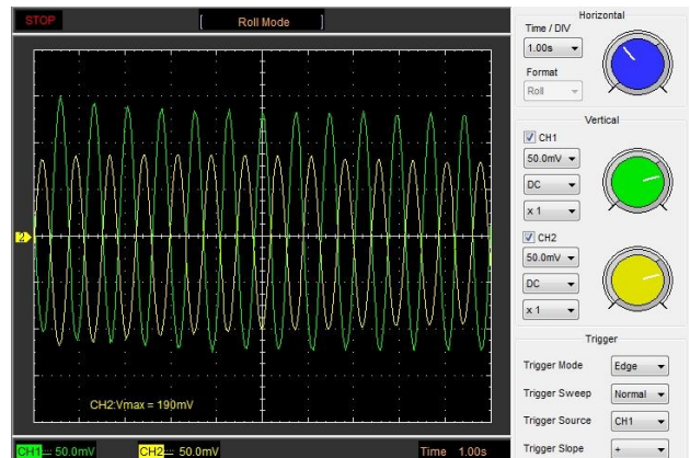
Fig. 8: Oscillation components for a string pendulum swinging along the line perpendicular to that bisecting the two force sensors
