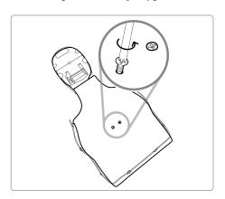
1) Disassemble two screws from the back of the manikin. If the screw are not installed on your version please proceed to the next step.
