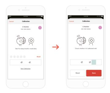
5) When the kit is connected to the app for the first time, the breath sensor should be calibrated. The calibration screen will pop up automatically.
