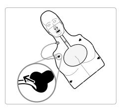
3) When assembling chest frame back to the manikin, do not forget to pass the breath module through the left top hole on the chest frame
