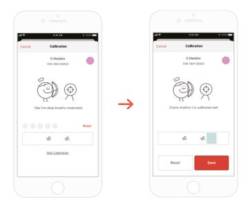
3) When the kit is connected to the app for the first time, the breath module should be calibrated. The calibration screen will pop up automatically.
