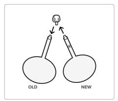
2) Remove the lung bag which is not equiped with the Breath module holder and install the new lung bag delivered in the Upgrade kit.
