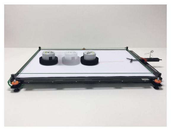
Sample experiment: Elastic collision
