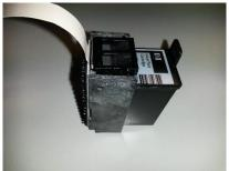
2. Pass the connector through the window of the L-bracket with Velcro, then velcro the cartridge holder in the L-bracket.
