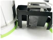
4. Slide the assembly with ink cartridge into the rectangle.
