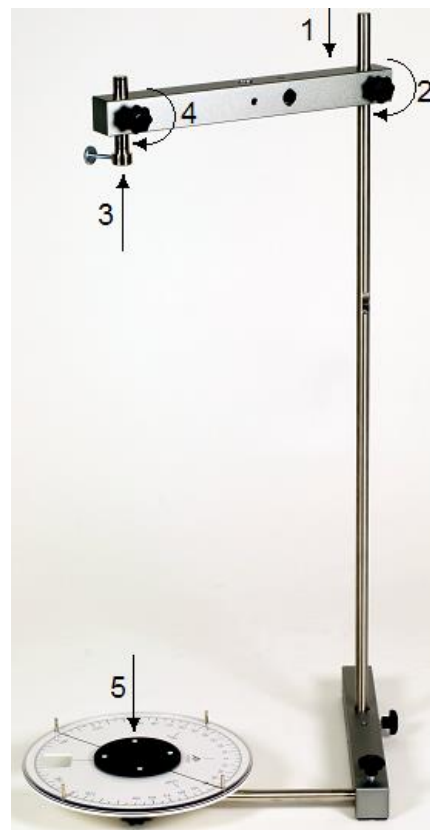
Fig. 4: Assembly of upper cross piece (wire of length 500 mm), clamping sleeve and pendulum disc.
