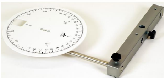
Fig. 2: Assembly of scaled disc with horizontal rod and cross piece.
