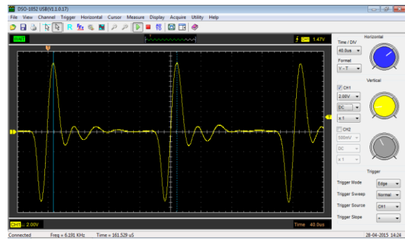
Fig. 2 Oscillation pulses in a 400-mm stainless steel rod struck with a pulse-like beat.
