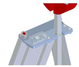
Fig. 2: Bearing plate with pendulum rod suspended
