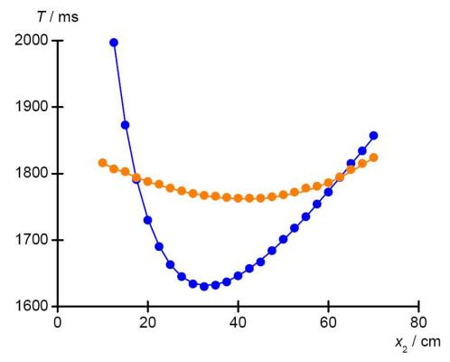
Fig. 6: Period of oscillation T as a function of the distance  $x_2$  of the moving pendulum bob from the suspension point (the bearing fulcrum). Red circles: Both pendulum bobs below fulcrum. Blue circles: Fixed pendulum bob above fulcrum, movable bob below
