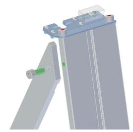
Fig. 1: Attachment of stand rod to stand board
