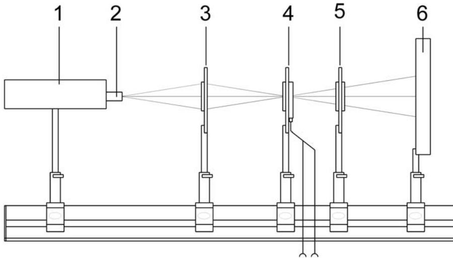
Fig. 4 Set-up for demonstrating birefringence from an  $\text{LiNbO}_3$  crystal.
