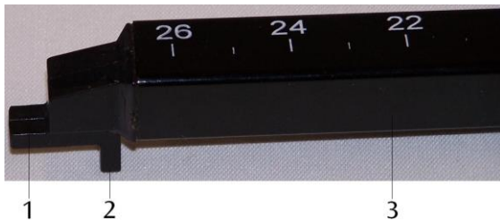
Magnetic field probe: 1 tangential Hall probe (z-direction), 2 axial Hall probe (x-direction), 3 probe carrier
