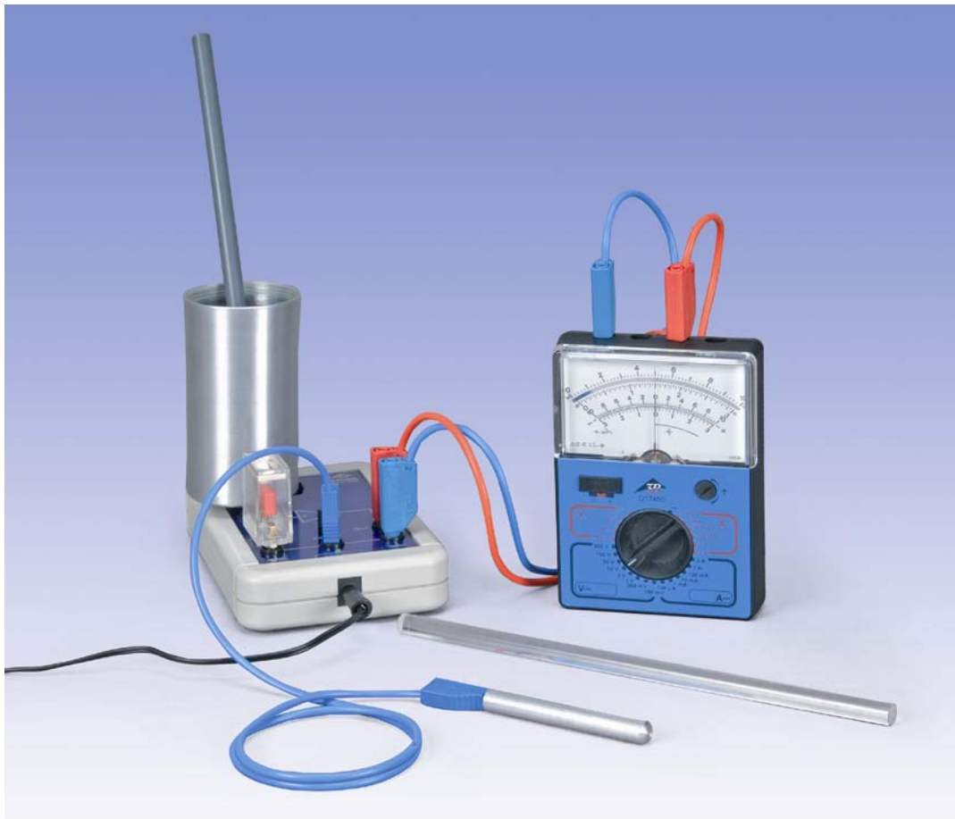
Fig. 1 Experiment set-up for measuring charges in electrostatics
