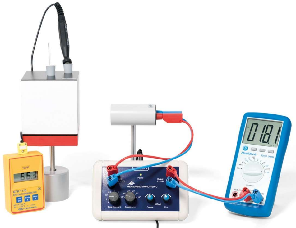
Fig. 1: Experimental set-up Leslie's cube
