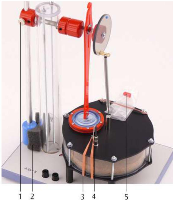
Fig. 7: Stirling engine as secured for storage
