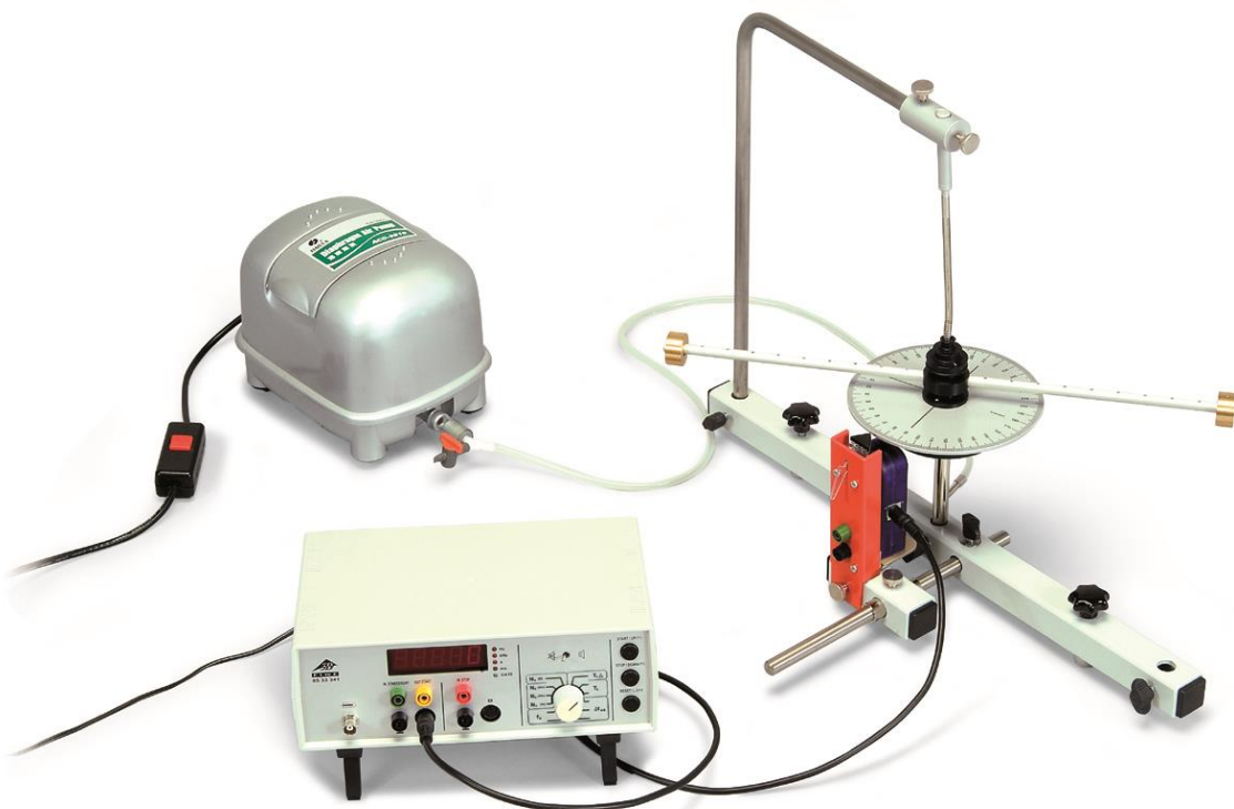
Fig. 2 Experiment set-up for determining moment of inertia of transverse beam with additional masses, using a laser reflection sensor (1001034) and a digital counter (1001032 or 1001033).
