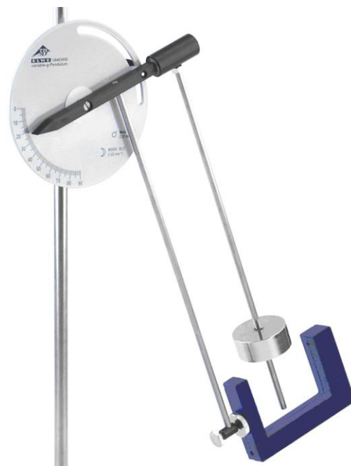
Fig. 1 Variable-g pendulum with mounting rod and photo gate
