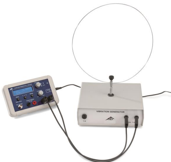
Fig. 3 Experimentel set-up with the resonance wire
