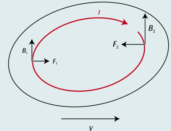
Eddy current  $I$  in a metal disc moving at speed  $v$  through a uniform magnetic field  $B_1, B_2$  with Lorentz forces  $F_1$  and  $F_2$  acting on both limbs of the eddy. The force acting against the motion is greater than that operating in the same direction.
