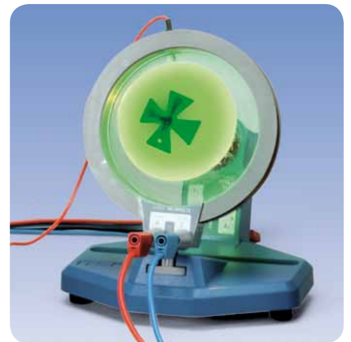
Fig. 2: Rotation of the electron shadow through deflection of electrons in the axially aligned magnetic field.
